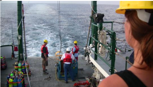
Crew preparing to deploy side scan-sub bottom profiler towfish
